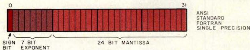
Figure 1: The American National Standards Institute (ANSI) floating point format for FORTRAN. It consists of a 24 bit mantissa, a 7 bit exponent and a sign bit.
