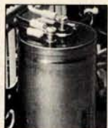
OVERSIZE CAPACITORS 280,000 uf FILTER CAPACITANCE -8V 43,000 uf FILTER CAPACITANCE ON EACH ± 16V dc
